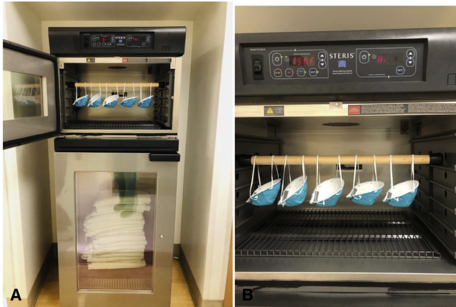
Figure 1. (A) Use of a hospital blanket warmer to heat N95 masks to 70°C (158°F) for 60 min. (B) There may be other, better methods to hang N95 masks, but note that masks may need to be > 6" from the walls of the heater to prevent mask degradation, depending on the temperature of the surface of the walls.
