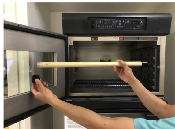
Figure 2. Assembly of a wooden dowel with end caps used to hang N95 masks.
